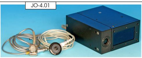
JO-4.01 was a passive infrared set with a range of about 500m. It was the successor of the 'Rostock' and operated in combination with a JO-4.02 or JO-4.03 at the other side of a link. Though originally used for transmitting in one direction only, optionally a separate receiver unit (left) could be bolted to the left hand side allowing two way conversation, primarily for use by agents.
