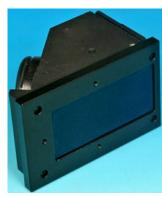
Mirror and diaphragm assembly of the JO-4.01. When placed behind a window pane it could transmit conversations in that room.
